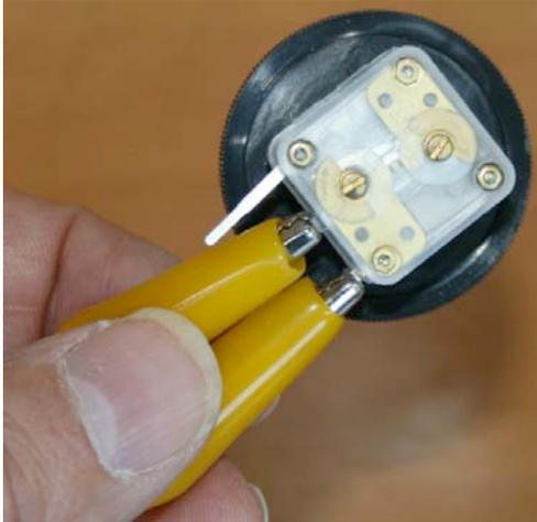
2. **Test lead clip #2:** Attach one clip to the same end of the box coil, and the other side to the center terminal of the variable capacitor (connections are made with the dial facing away from you).
